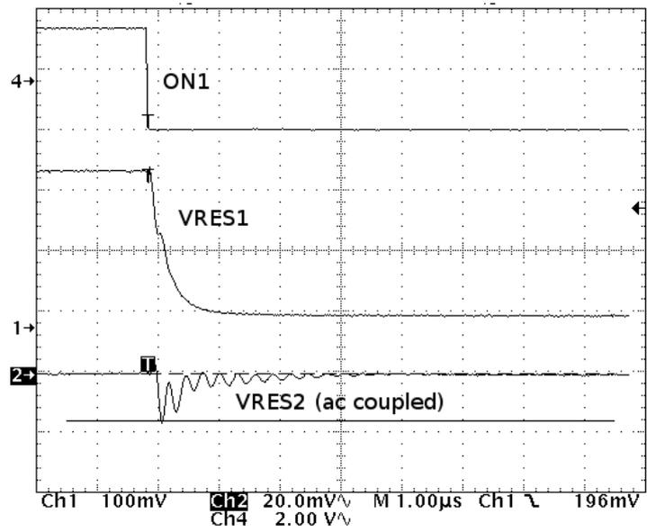
Figure 10 – PWM performance of Current Source CURR1, I(CURR1) changed between 400mA (ON1=1) and 20mA (ON1=0); AS3691A
