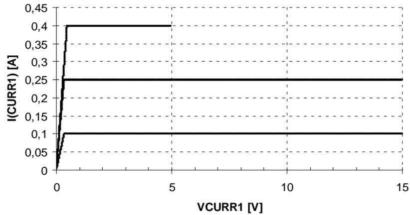
Figure 6 – Output Current versus Voltage on Current Source – Low Current Range
