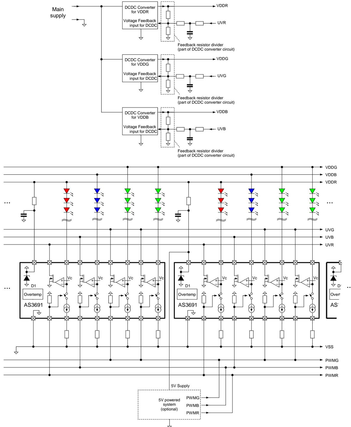
A typical AS3691 for single color leds can be done as follows using automatic supply regulation (feedback path UV):
