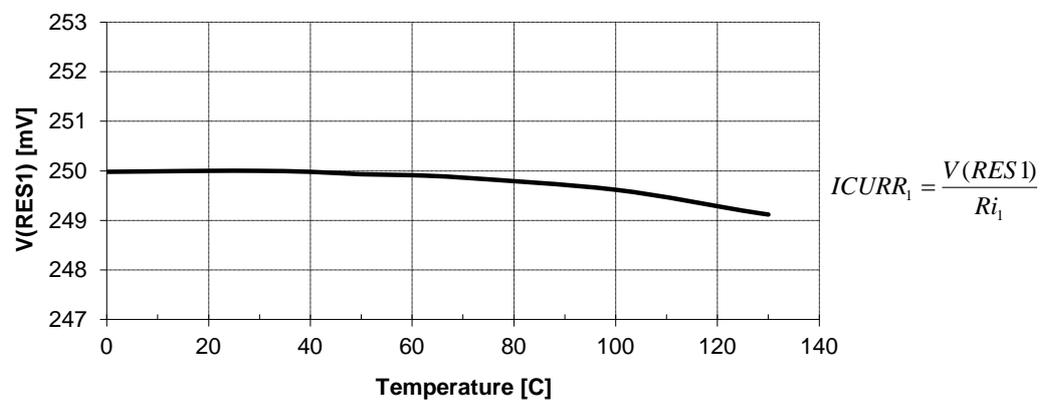
Figure 8 – Output Current versus Temperature,  $V(\text{CURR1}) = 2.0\text{V}$ ,  $R_{i1} = 2.5\Omega$  (Note: temperature coefficient of  $R_{i1} = -200\text{ppm}/^\circ\text{C}$ )
