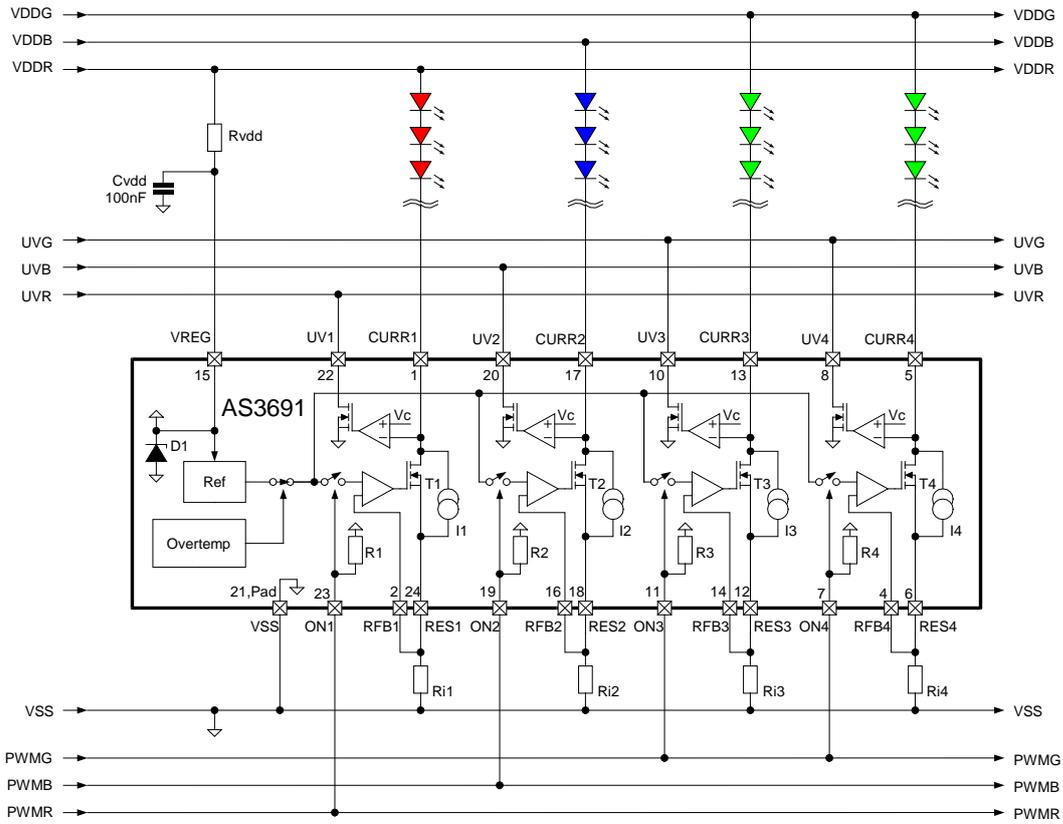
Figure 3 – Complete AS3691 Application using White LEDs
