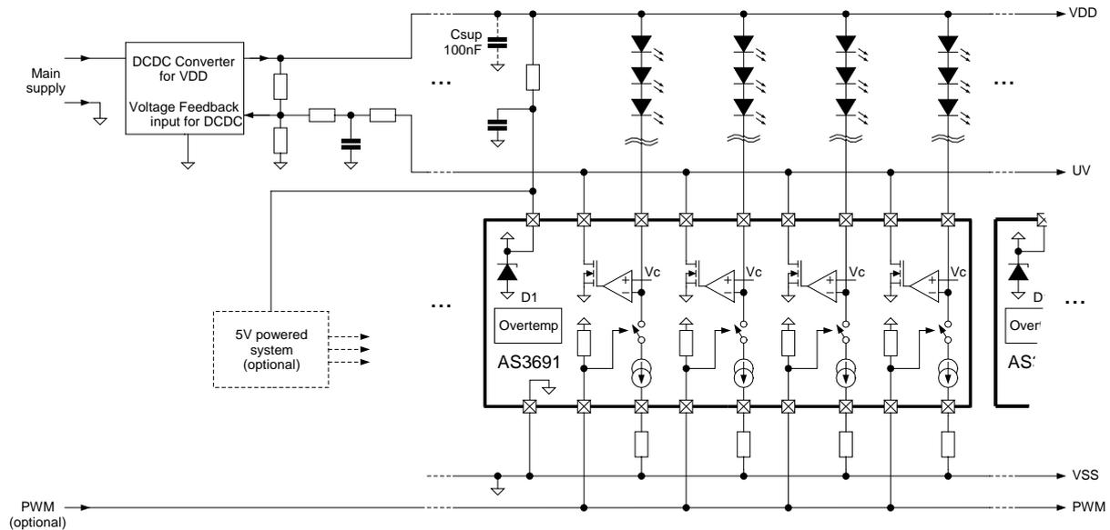
Note: Csup (100nF) is only required, if there are long wires (>0.3m) between the DCDC converter and the AS3691. The wire length between the Csup capacitor and the CURRx pin on AS3691 should not exceed 0.3m. If this cannot be guaranteed, add additional capacitors of 100nF to the pins CURRx.
