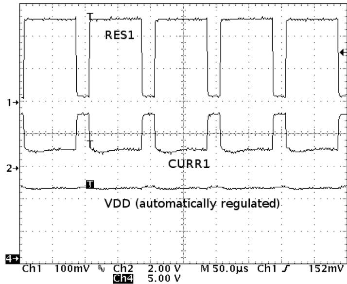
Figure 13 – Parallel Current I1 to I4 (for measurement of I1 remove current set resistor R1)
