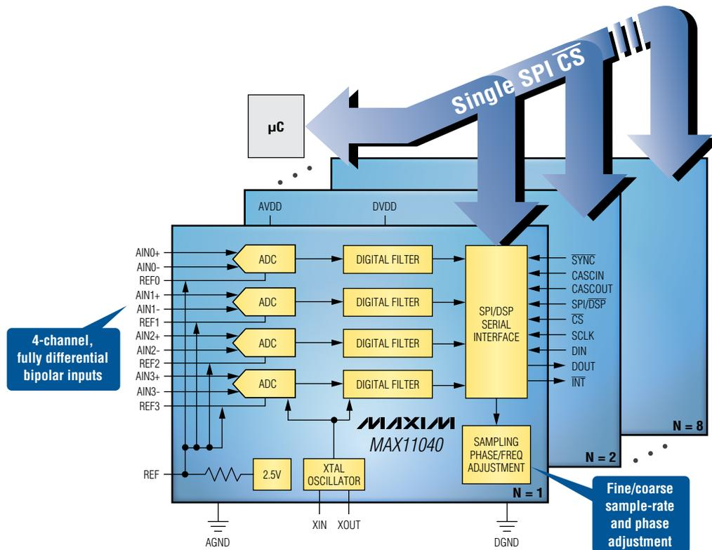
The MAX11040 can be cascaded up to 32 simultaneous channels.
