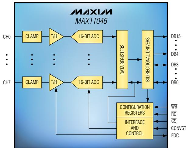
Block diagram of the MAX11046 16-bit, 8-channel, simultaneous-sampling ADC. Eight inputs measure voltage and current signals on three phases plus neutral.
