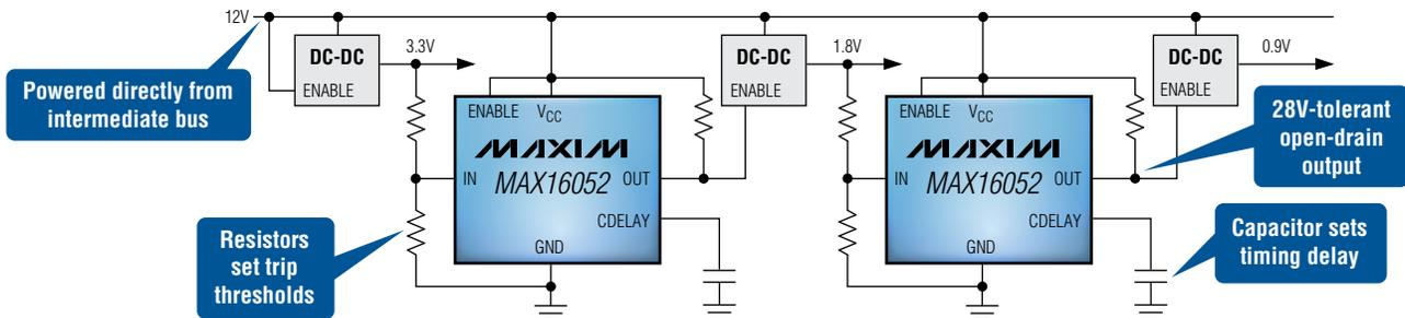
The MAX16052 in a typical monitoring application.
