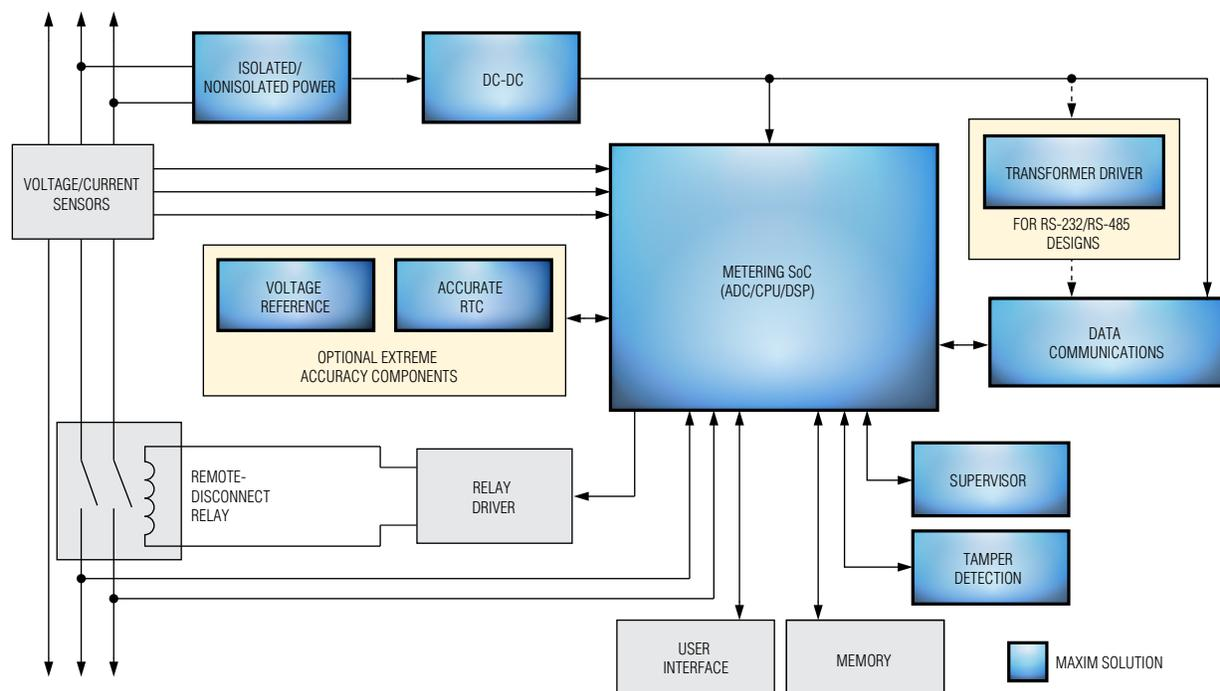
Smart meter block diagram. For a list of Maxim's recommended smart meter solutions, please go to: [www.maxim-ic.com/smartmeter](http://www.maxim-ic.com/smartmeter).
