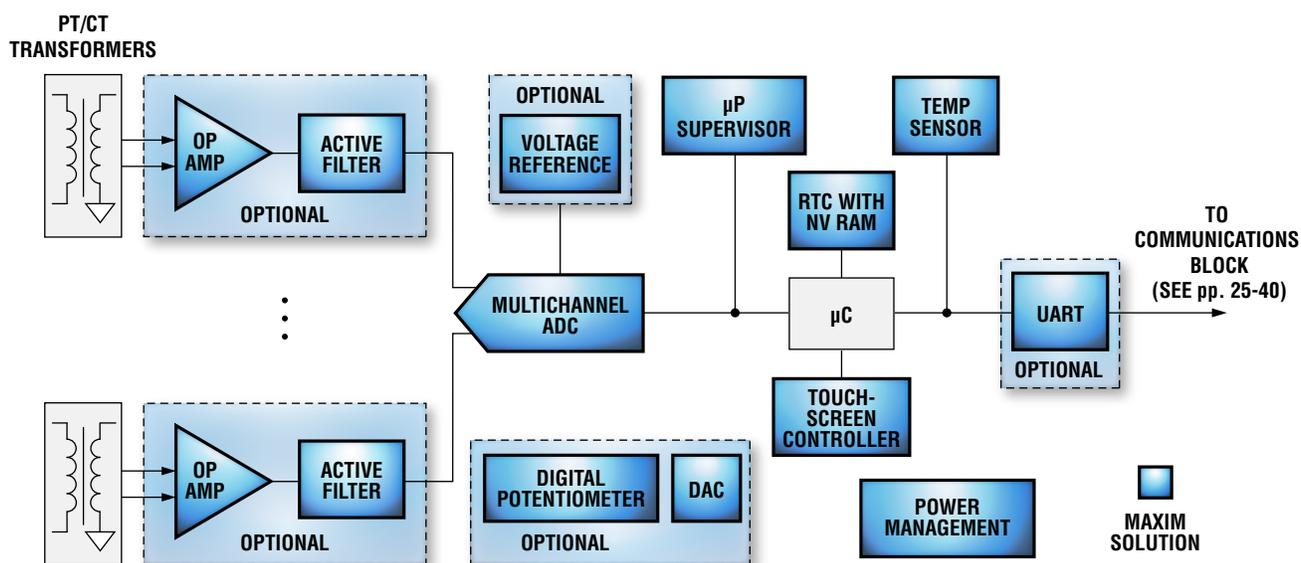
Block diagram of a typical power-grid monitoring system. For a list of Maxim's recommended power-grid monitoring solutions, please go to: [www.maxim-ic.com/grid-monitoring](http://www.maxim-ic.com/grid-monitoring).
