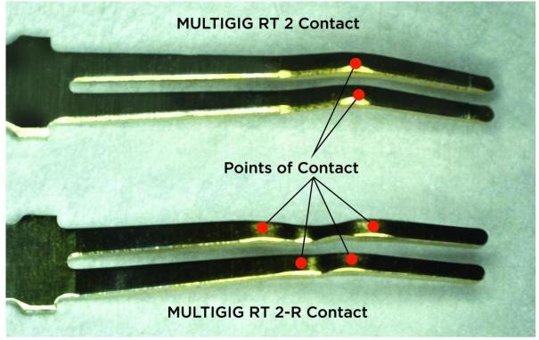
Figure 3. Original and quad redundant MULTIGIG RT 2 contacts
