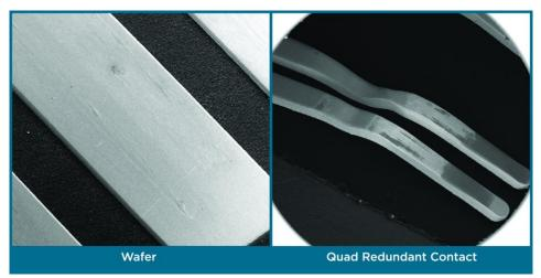
Figure 5. Contacts after 10,000 mating cycle durability testing show acceptable contact surfaces.
