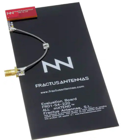
Figure 6: The Ignion antenna evaluation boards include a grounded 50 \Omega micro-coaxial cable which can be connected to a network analyser.
