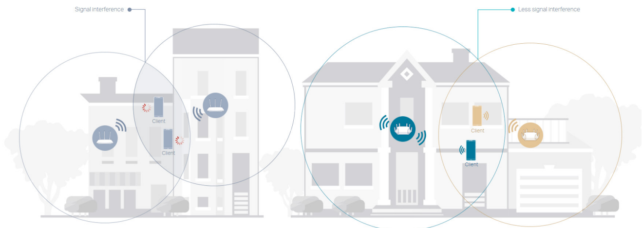
Figure 3. A diagram that shows a reduction in overlapping basic service set interference with Wi-Fi 6's BSS colouring feature. Credit: tp-link
