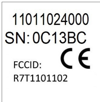
Figure 5: Example of an ID label appended to the Setebos-I module to show that it has passed CE and FCC RF certification. Certification can generally be inherited by the end product without retesting through some simple paperwork. Image source: Würth Elektronik
