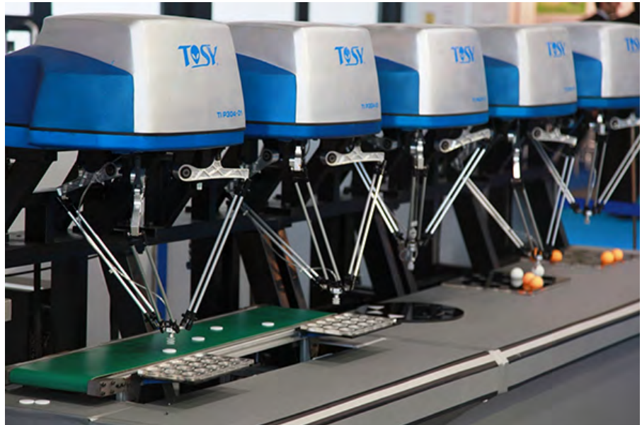
Figure 2: A delta robot is a type of parallel manipulator with three parallelograms all connected to a single rigid body at the end effector end. The base of each parallelogram is actuated in a single degree of freedom relative to the robot's base. Delta robots are typically ceiling mounted to tend conveyors or workpieces from above. (Image source: Wikimedia Commons)
