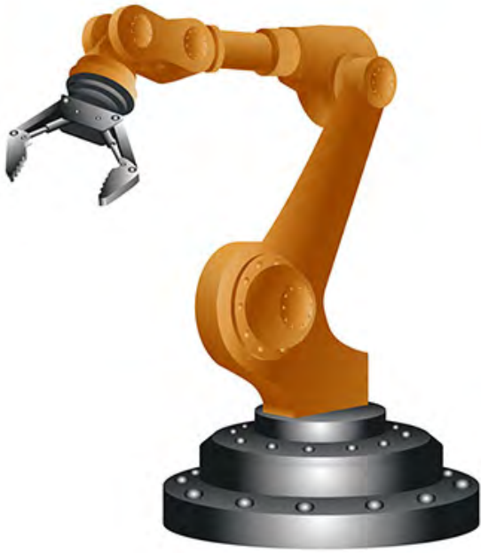
Figure 1: Shown here is a two-finger pneumatic gripper on the end of a robotic arm. The jaw fingers make physical contact with the object to be grasped and are what allow the gripper to hold and release objects. (Image source: Kazakov • Getty Images)
