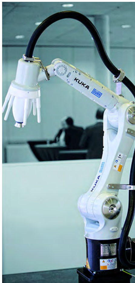
Figure 5: Compact industrial robots that are complete system solutions for common applications are now available "off-the-shelf", such as this painting system from Dürr Group and KUKA Robotics. (Image source: Dürr AG)
