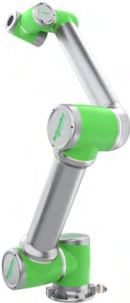
Figure 2: This cobot can move 12 times faster than the maximum allowed by ISO/TS 15066 when a person is in the collaborative workspace. (Image source: Schneider Electric)
