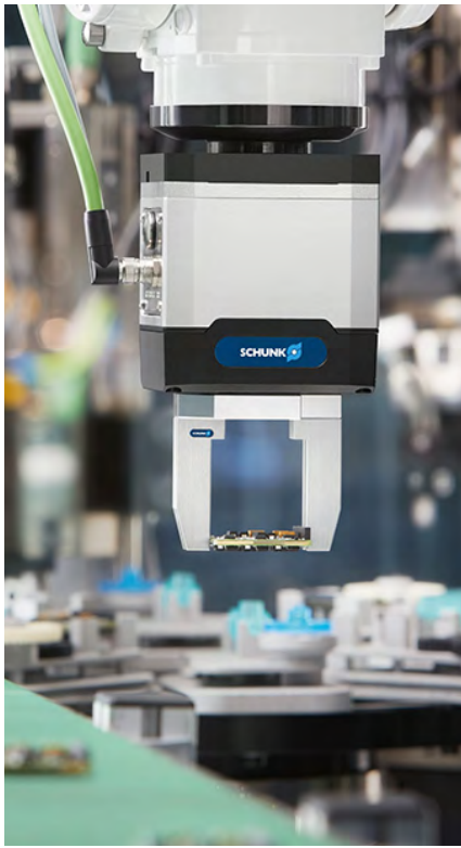
Figure 4: Small-component EGK grippers are lubricated with H1 grease and sport cleanroom certification. (Image source: SCHUNK Intec Inc. )
