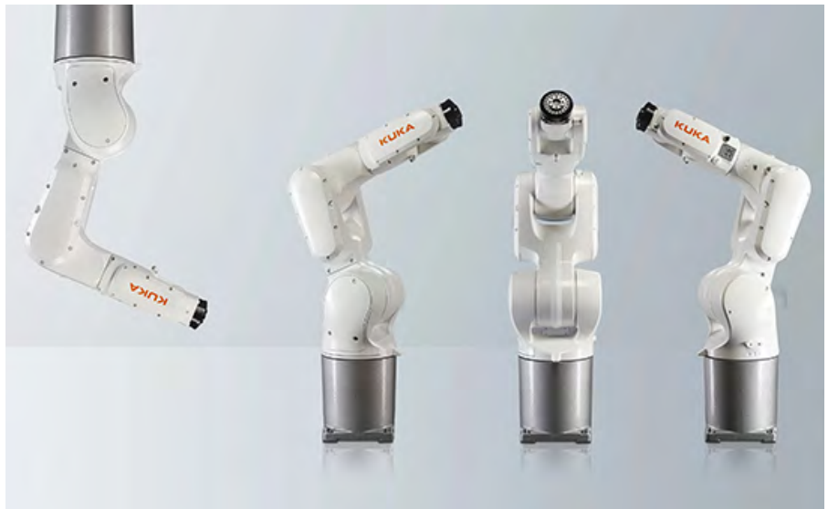
Figure 5: These six-axis robots are what most people picture when imagining an industrial robot. (Image source: Kuka )
