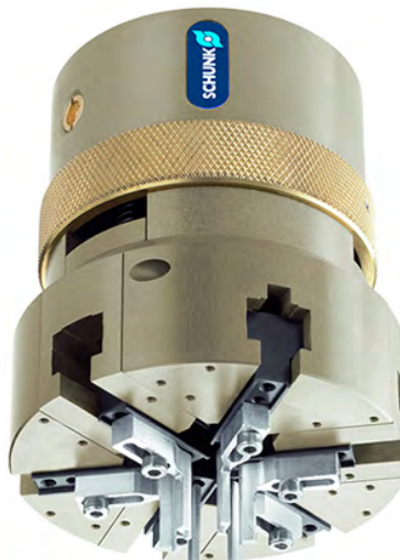
Figure 2: Parallel, three-finger, and angled grippers are the three most common gripper types in industrial applications. The three-finger pneumatic gripper shown here has fingers offset by 120° to gently stretch O-rings and mount them onto recipient shafts. (Image source: Schunk)
