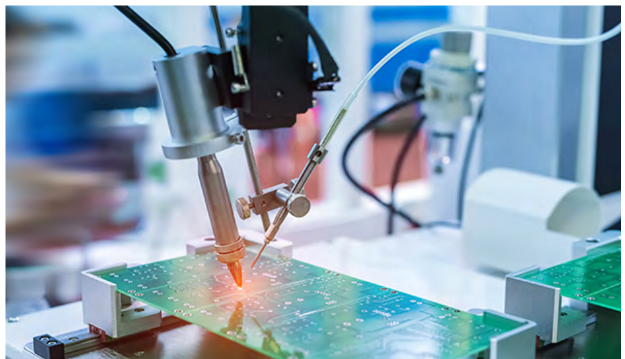
Figure 6: Robotic end effectors can take the form of soldering iron tips to automate the assembly of subcomponents onto PCBs. (Image source: Dreamstime)
