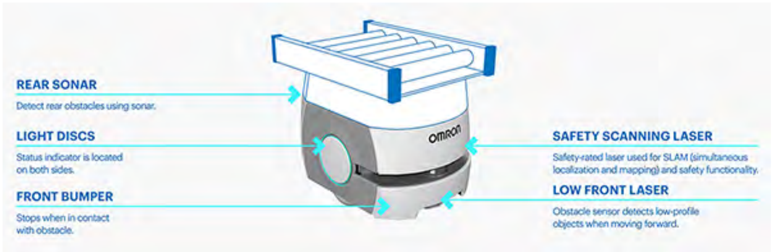
Figure 3: Type B AMR with a roller table attachment. This also shows typical navigation and safety systems common to all three types of AMRs. (Image source: Omron)
