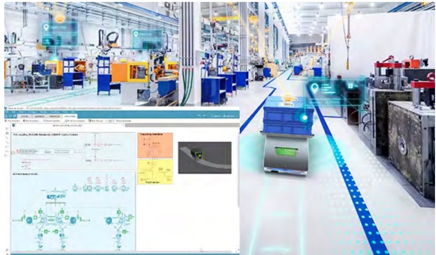
Figure 5: AMR digital twins can be virtually inserted into a simulated factory environment for virtual commissioning. (Image source: Siemens)
