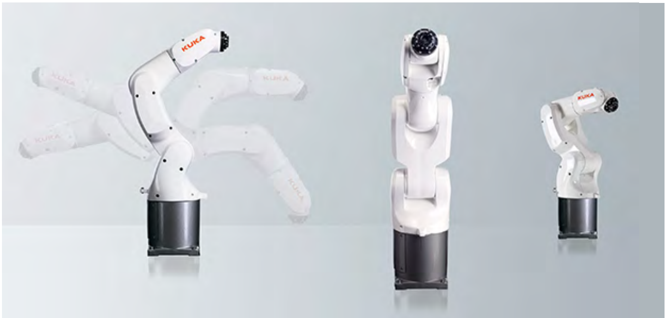
Figure 2: Manipulator arms, such as the AGILUS KR 3 R540 from KUKA Robotics, are bringing ROI for industrial robotics within reach of small to mid-size operations. (Image source: KUKA Robotics Corp.)
