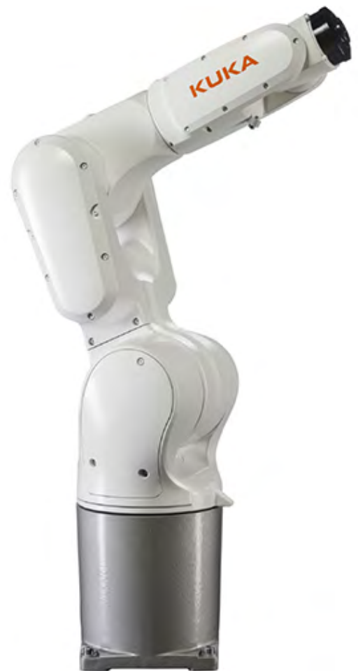
Figure 1: Six-axis articulated robot with a pose repeatability of \pm 0.02 mm. (Image source: DigiKey)
