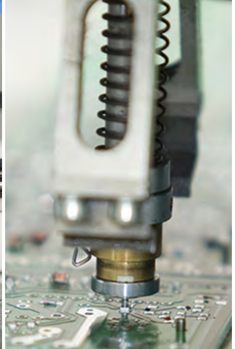
Figures 11a and 11b: Shown here are tool heads for affixing surface-mount technology (SMT) subcomponents to a board. (Image source: Dreamstime )
