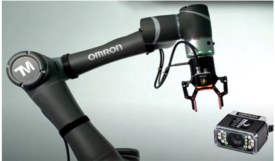
Figure 4: High-performance barcode readers can quickly and reliably decode 1D and 2D barcodes. Some mount on robotic end effectors to support part picking of electronic and automotive parts as well as subassembly elements. (Image source: Omron Automation and Safety )
