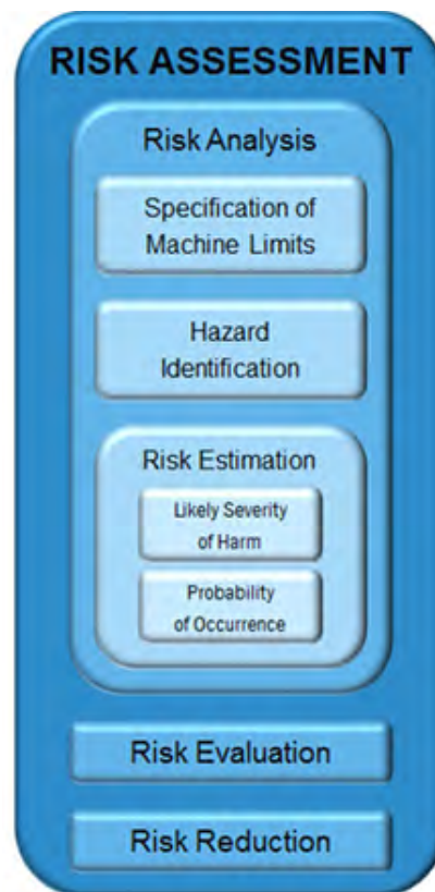
Figure 2: Key components of a risk assessment include risk analysis, evaluation, and reduction. (Image source: SICK )
