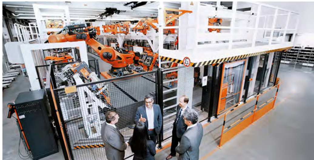
Figure 1: Traditional industrial robots tend to be large and fast-moving, requiring protective cages to ensure worker safety. (Image source: KUKA Robotics Corp.)
