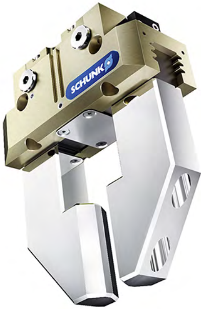
Figure 3: Two-finger parallel grippers in Schunk's PGN-plus series deliver long jaw strokes and include seals, dirt-resistant round linear guides, and high-strength aluminum-alloy housings to survive dirty industrial environments. (Image source: Schunk)
