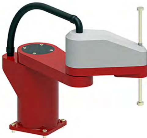
Figure 7: SCARA robots execute pick-and-place wafer handling and processing tasks quickly and precisely. (Image source: Dreamstime)
