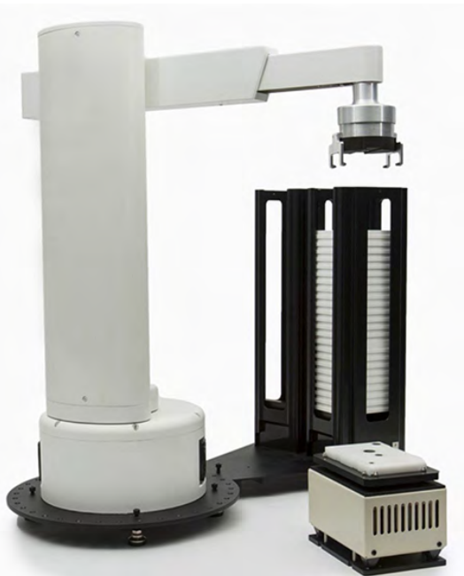
Figure 3: This cylindrical robot has one rotary and prismatic joint. (Image source: Association for Advancing Automation)
