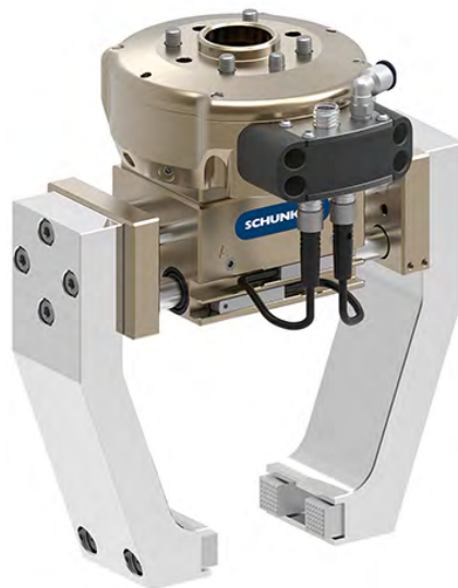
Figure 3: Two-finger parallel grippers in Schunk's PGN-plus series deliver long jaw strokes and include seals, dirt-resistant round linear guides, and high-strength aluminum-alloy housings to survive dirty industrial environments. (Image source: Schunk)
