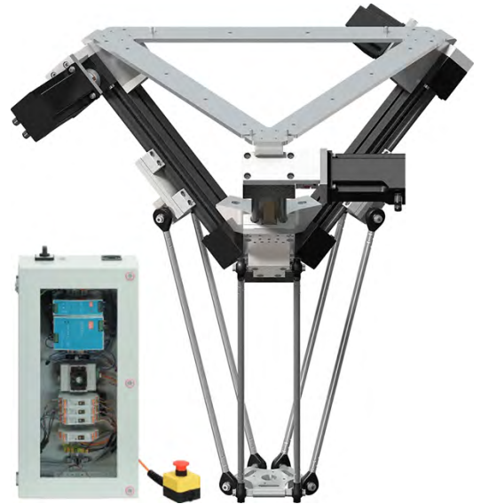
Figure 4: Three-axis delta robot and controller (left). (Image source: DigiKey)
