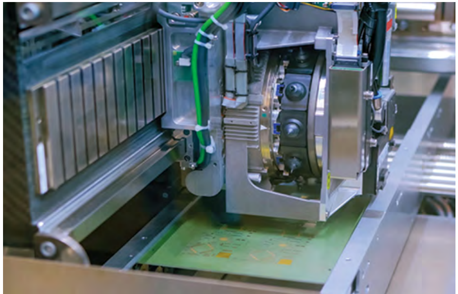
Figure 9: Cartesian robots execute fully automated semiconductor manufacturing tasks. Note the linear motors that provide high-precision direct driving on the critical axis. (Image source: Dreamstime)
