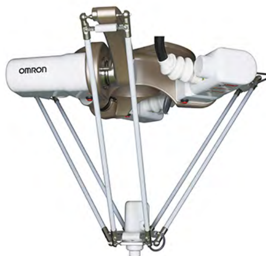
Figure 4: This servomotor-driven delta robot moves to 200 cycles per minute in three degrees of freedom (DOFs) plus a rotational axis. A controller can command these robots' axes with 2-msec response time to synchronize with conveyors and other tasks. In fact, another delta-robot is the Quattro; it has four instead of three parallelograms connecting the base to the end effector to deliver high stiffness and positioning accuracy at high speeds. (Image source: Omron Automation )
