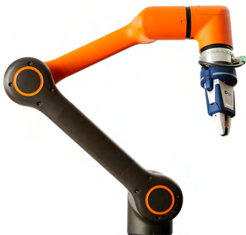
Figure 13: Cobots in the HCR-5 series meet ISO-2 cleanroom specifications. (Image source: Hanwha Corp./Momentum )
