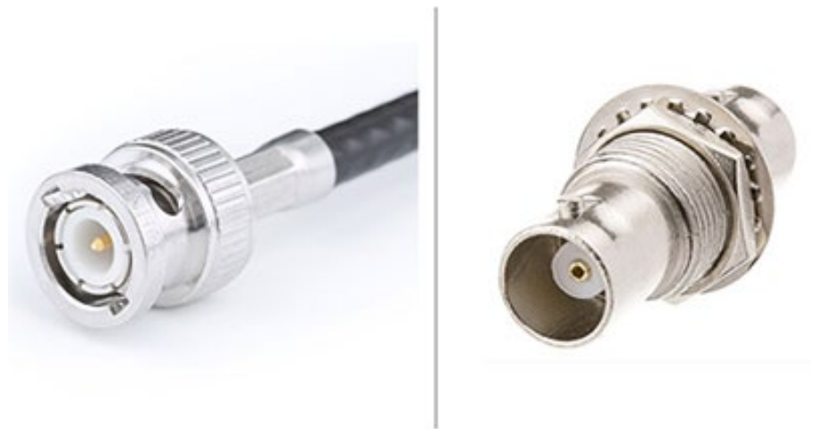
Figure 1: The BNC connector includes a bayonet body lock and has been widely used since its development in the early 1950s, but it is not a good electrical or mechanical fit for many of today's high-frequency, space-constrained applications. A male plug is usually used with cable assemblies (left); a female jack (right), for use on instrument panels. (Image source: Wikipedia; Pinterest)
