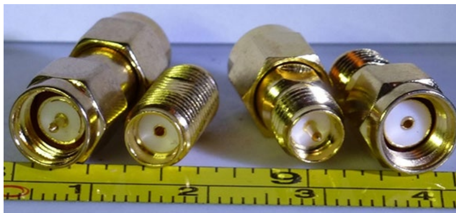
Figure 13: RP SMA plug and jack connectors have the opposite center conductor gender compared to conventional SMA connectors; (left to right) standard SMA male connector, SMA standard female connector, RP-SMA female connector, RP-SMA male connector. (Image source: Wikipedia)
