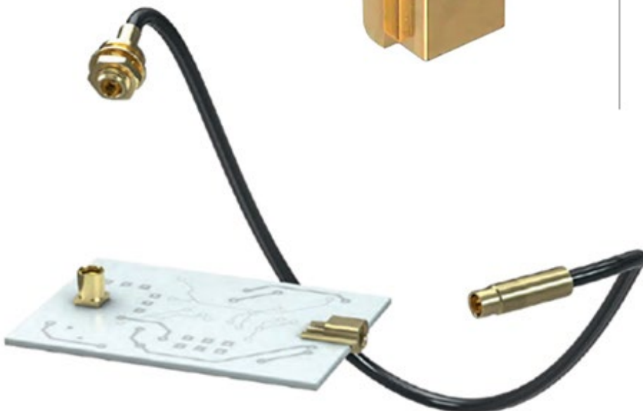
Figure 10: Connectors in the MMCX series are approximately 30% smaller than those in the MCX series and exhibit comparable RF performance. (Image source: Würth Elektronik)
