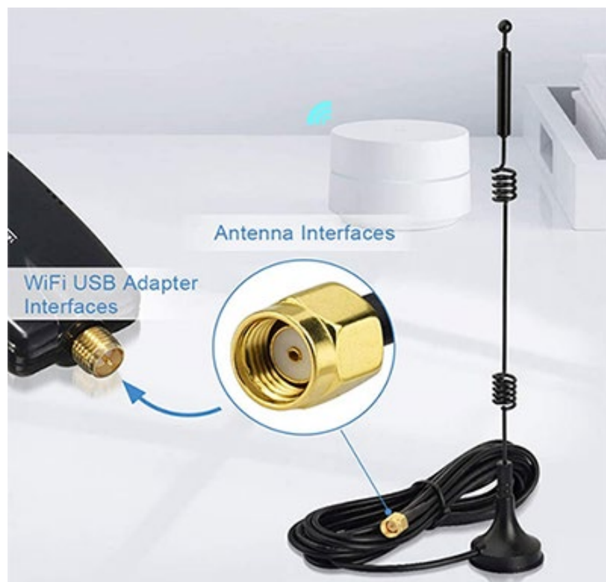
Figure 14: This external Wi-Fi antenna can be moved around to find an optimal location and is connector compatible with the antenna interface on the Wi-Fi router due to its RP-SMA connector. (Image source: Amazon)
