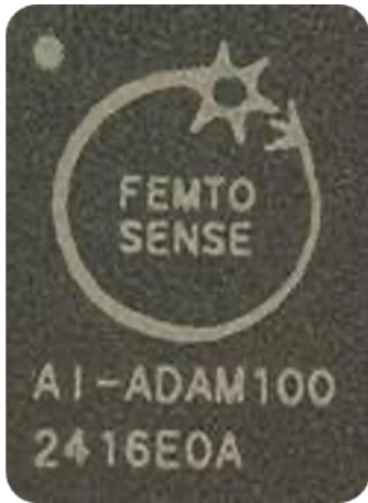
Figure 2: Combining a sparse neural network accelerator with an ARM microcontroller in a single package
