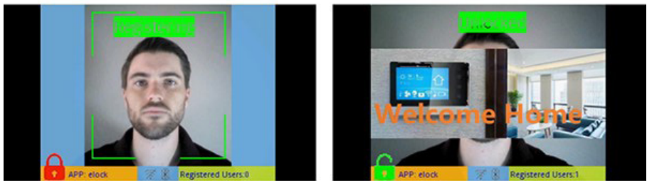
Figure 6. The NXP SLN-VIZNAS-IOT hardware kit works out of the box, utilizing a companion app to register a face (left) and recognize registered faces (right). Image source: NXP
