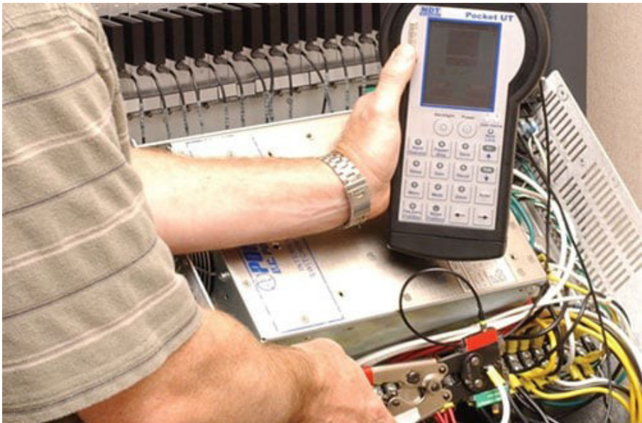
Figure 8: This portable instrument developed by NASA can non-destructively identify both good crimps and the many types of bad crimps in real-time. Image source: NASA
