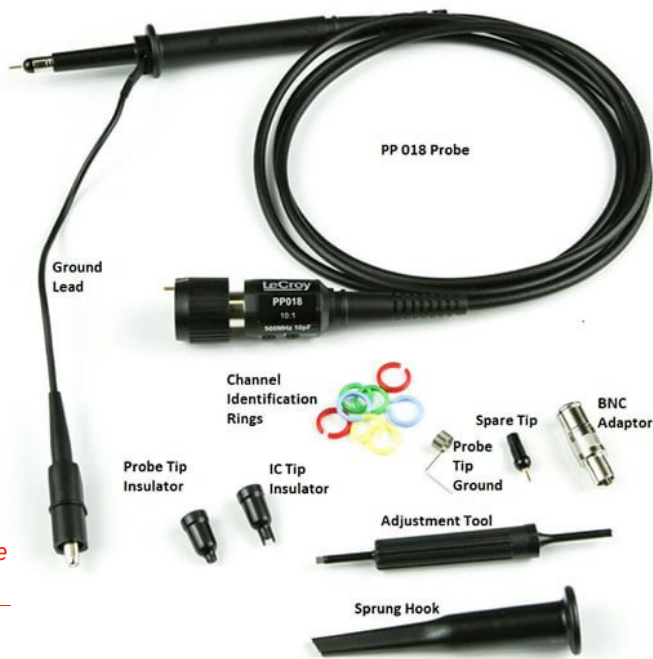
Figure 2: The PP018 high impedance probe has a bandwidth of 500 MHz and an input capacitance of 10 pF. It is shown here along with supplied accessories.
