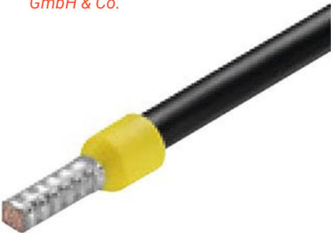
Figure 3: This crimped wire-end ferrule is available in many sizes and has a plastic collar as an additional insertion aid due to the conical shape in the inner diameter of the collar. Image source: Weidmüller Interface GmbH & Co.
