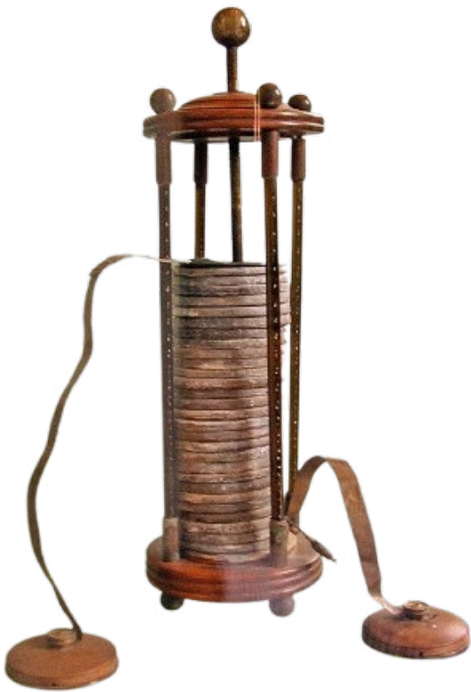
An example of an early Voltaic pile.
