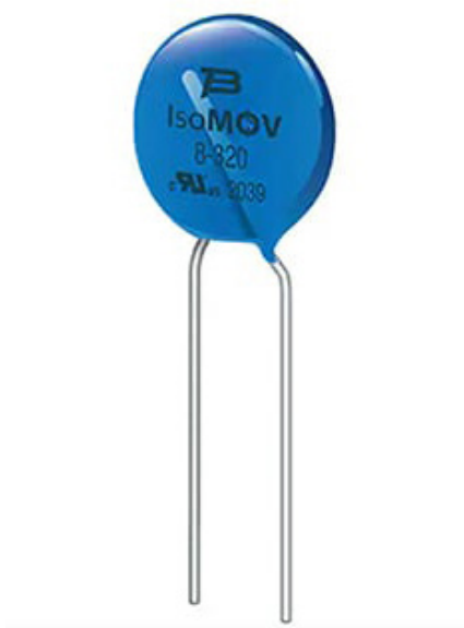
Figure 5: The ISOM3-175-B-L2 is an example of the IsoMOV hybrid protector's compact form factor. Although it includes two MOVs and a GDT, it measures just 13.2 mm in diameter with a thickness of 6.1 mm. (Image source Bourns)
