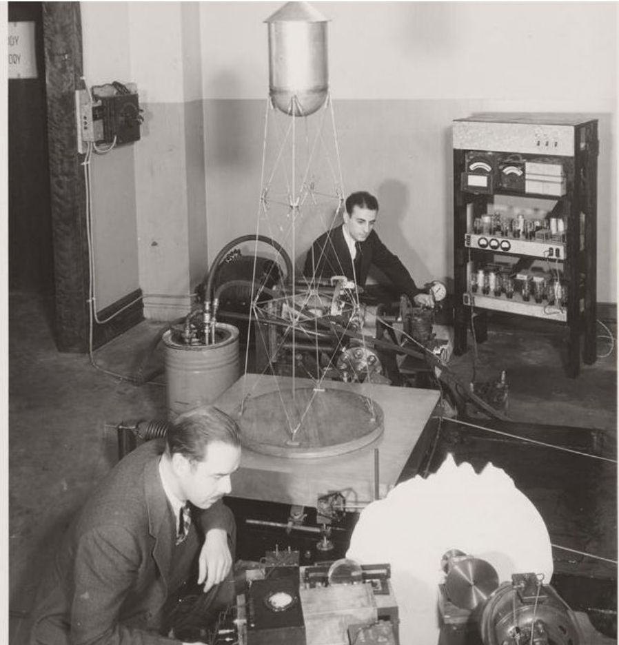
Ruge and his assistants solving structural stress problems with a model of a water tower. This is likely the same problem that he was working on when he developed the strain gauge.
