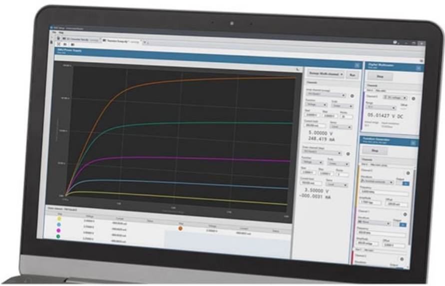
Figure 4: InstrumentStudio can present data from multiple instruments on one screen. For example, from an oscilloscope (large left panel), a DMM (top right panel), and a function generator (bottom right panel). Source: NI
