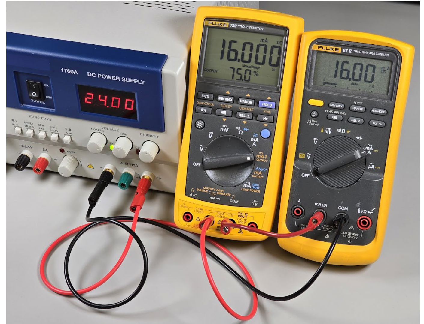
Figure 1: Image of the process meter configured for transmitter mode simulating a sensor operating at 75% of span which corresponds to 16 mA.
