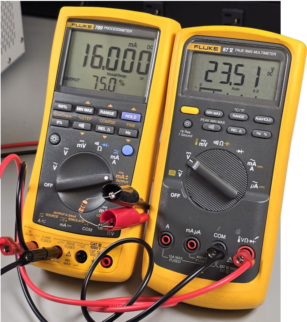
Figure 3: Process meter configured for source mode driving a 1.5 k \Omega load resistor. Source: DigiKey
