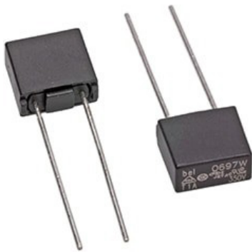
Figure 3: The 0697W series are AEC-Q compliant, radial lead, high voltage, time-lag fuses. Image source: Bel Fuse
