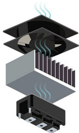
Figure 3: Utilizing heatsinks and fans represents a highly effective thermal management solution for IGBTs. Image source: Same Sky
