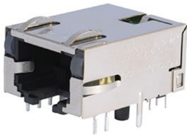
Figure 5: The MagJack automotive Ethernet single-port ICMs feature integrated magnetics to meet the need for compact solutions. Image source: Bel Fuse
