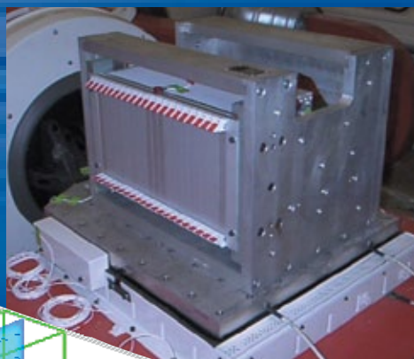
Subrack shock and vibration test
