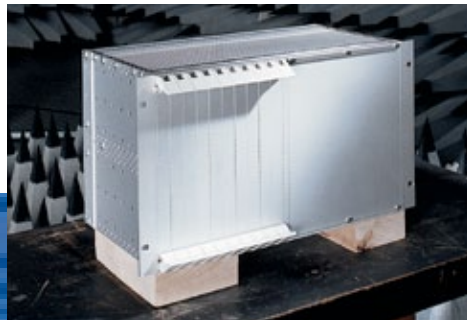
Subrack electromagnetic shielding performance test
