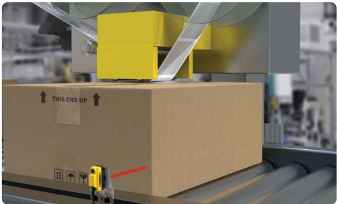
Single-Point Leading Edge Detection
