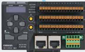
IO-Link Master Unit GD Series
