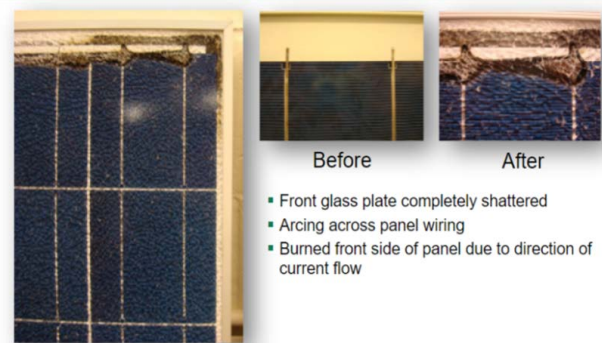
FIGURE 3. Polysilicon panel failures include glass destruction, arcing and burning of panels
