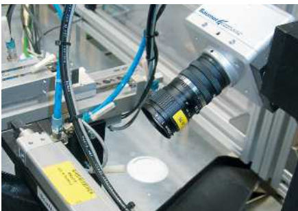
Quality inspection using optical camera systems
