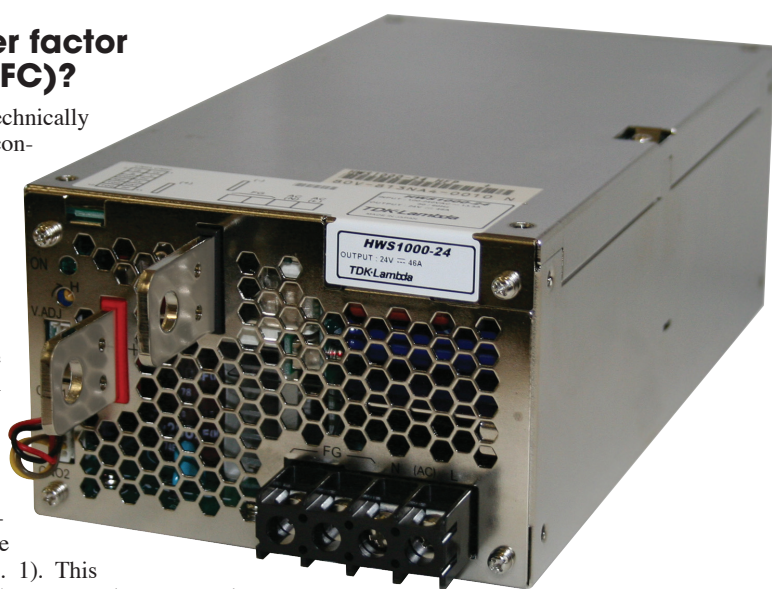
Typical 1000-Watt Switchmode Power Supply with PFC (meets EN61000-3-2) Power Factor = .98, Efficiency = 88%
