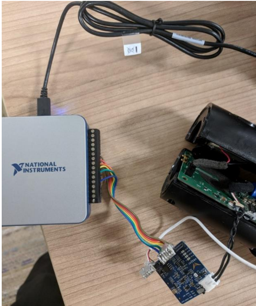
Figure 11: completed wiring for current monitoring
