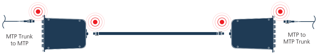
MTP to MTP trunk design required with 4 mated pairs , a total of 2dB connector loss
