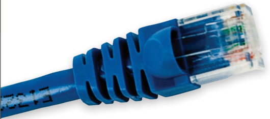
Category 6 Patch Cords Category 6 patch cords offer a slim-line boot. This molded strain-relief boot helps prevent tangling and excessive bending while reducing the stress on the cable.
