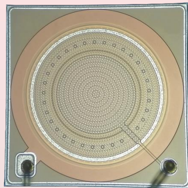
Magnified View of MEMS Microphone Diaphragm
