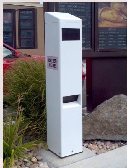
A Call Box Uses a Speaker as both a Microphone and a Speaker
