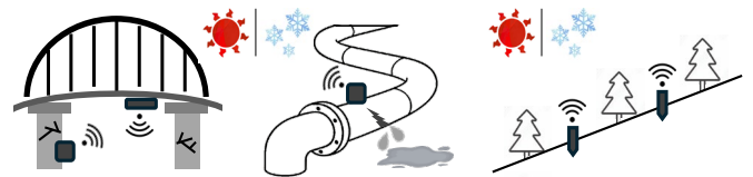
Figure 1. Example Use Cases: Strain and Vibration Sensors for Bridges, Vibration Sensors for Water Pipelines, and Landslide Monitoring Sensors
