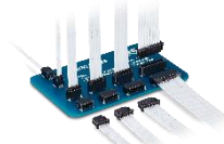
SignalBee™ KW30 Positive Lock (Center Lock) 1 Row Pitch: 1.0mm No. of Pos.: 2-15
