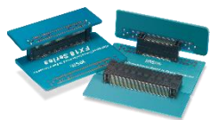
FunctionMAX™ FX18 10+Gbps High Speed Transmission Pitch: 0.8mm Stacking Height: 10-45mm No. of Pos.: 40-180* (*160, 180pos.: Coplanar Connection)
