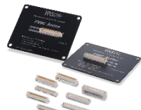
FunctionMAX™ FX8/FX8C 3.125Gbps High Speed Transmission Pitch: 0.6mm Stacking Height: 3-16mm No. of Pos.: 40-140
