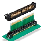
FunctionMAX™ FX27 Card Edge Connector Pitch: 0.8mm Stacking Height: 22mm Min. No. of Pos.: 40-120
