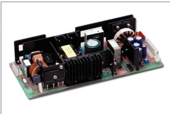
Figure 1: Photo of a convection-cooled (no fan) AC-DC switchmode power supply. Notice the black heat sinks, some of which have fins, while others are vertically mounted black sheet metal, which also serve as heat sinks to the high power devices used in the power supply circuits. This model (ZWD-PAF) is capable of providing up to 225-watts of output power with an ambient air temperature ranging from -10°C to +50°C.
