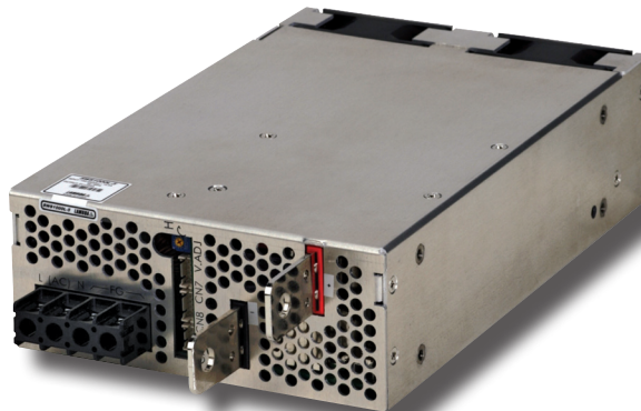
3. This unit, a SWS1000L series power supply, delivers up to 1 kW of output power and features alarm signals and active current sharing. Two or more can be connected in parallel with external isolation diodes to form a redundant and fault tolerant power system.
