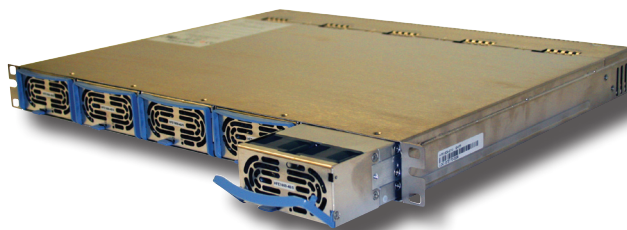
2. This HFE1600 series 19-in. rack-mount redundant power system houses five 1.6-kW hot-swap power supplies. If fewer supplies are required, blanking plates can be installed in the unused slots.
