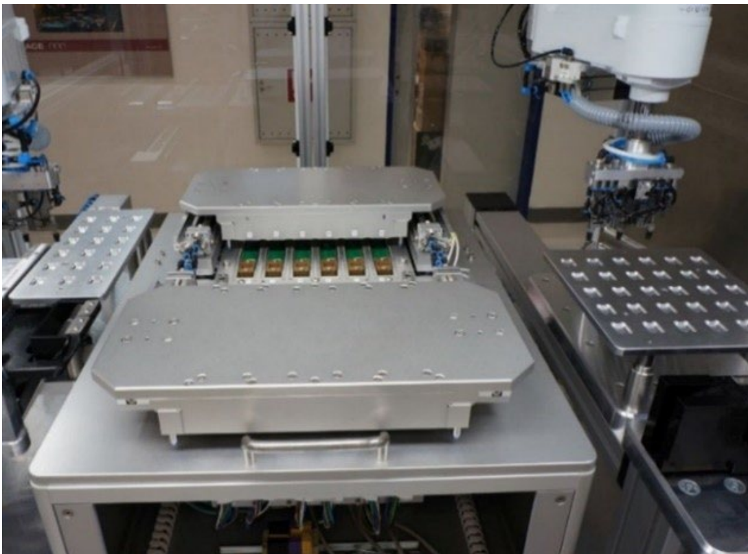
Figure 29: Automatic test equipment for module test
