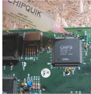
Apply Chip Quik® Tack Flux to all leads of SMD
