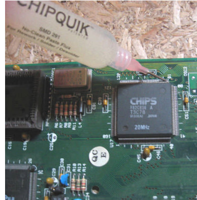
Apply Chip Quik® Tack Flux to all leads of SMD
