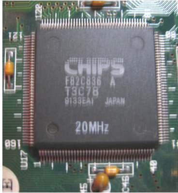
160 pin SMD to be removed with Chip Quik® SMD Removal Kit
