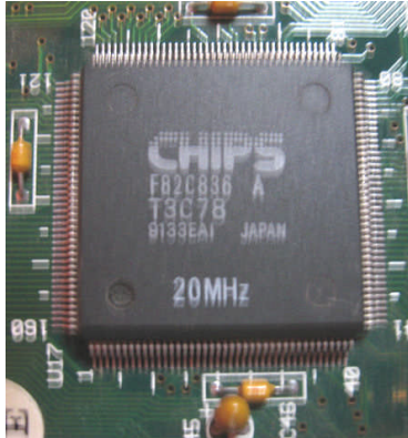
160 pin SMD to be removed with Chip Quik® SMD Removal Kit
