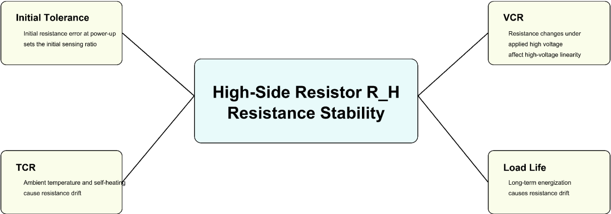
Figure 2. Main factors affecting high-side resistor stability
